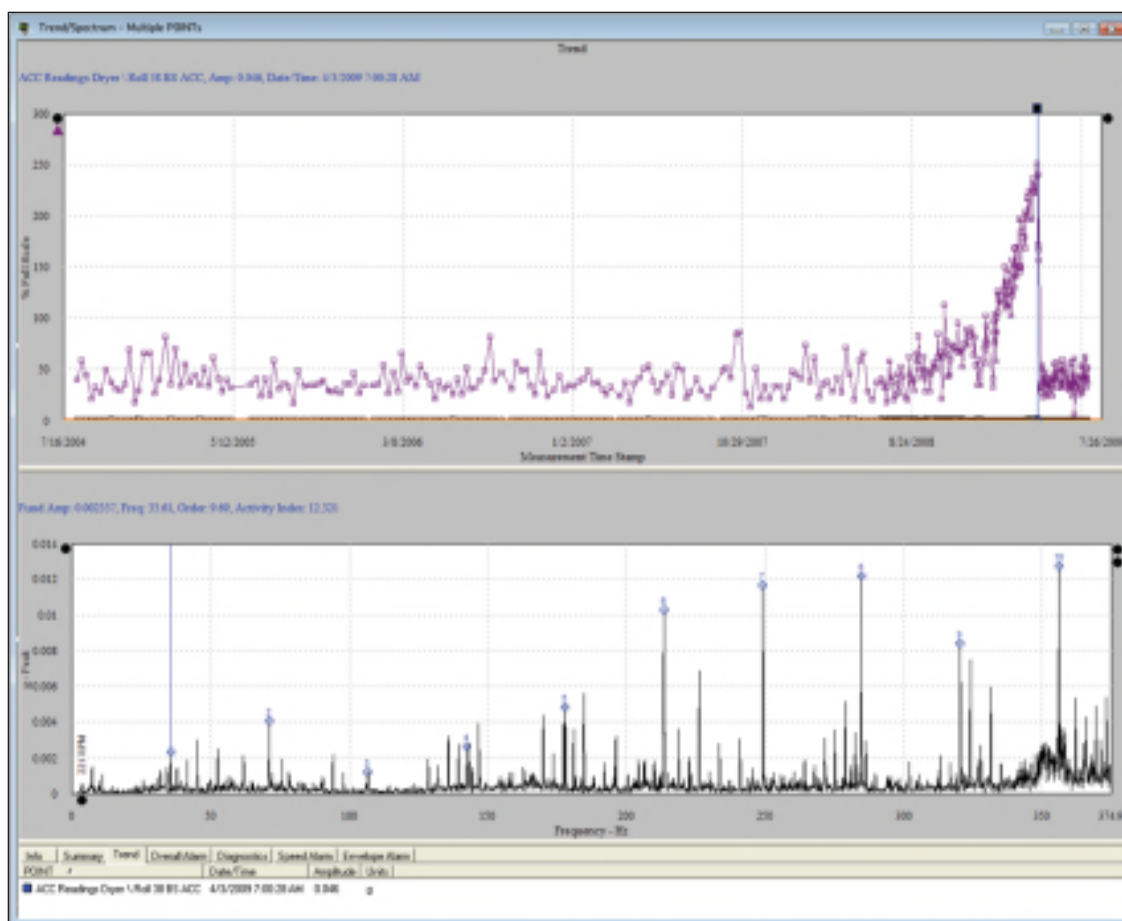
SKF @ptitude Analyst trend / spectrum plot.
