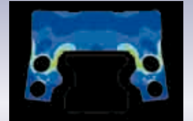
Example of roller slide deformation analysis
