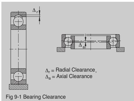
analyze the operating conditions to select appropriate amount of clearance for the bearings.
