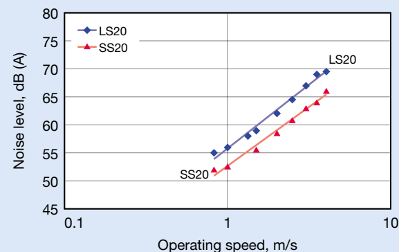
Fig. 2 Noise level comparison between LS20 and SS20
