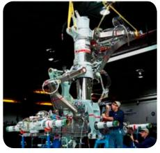
In the landing gear alone, SKF titanium bearings reduced weight by 40% for a 110 kg savings per plane. In the engine support frame and aileron flaps, they allowed a weight savings of an additional 90 kg per plane. The combined fuel savings of the titanium bearings for both position flaps and the landing gears represents close to 10 liters/hour of flight.
