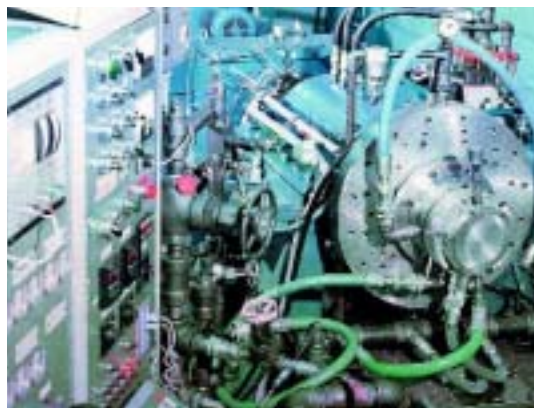
■ This Kaydon dynamic test rig (right) proved the pumping bushing seals, simulating Countrymark’s running conditions for the hydrogen compressor (left). A dynamic test report was provided for each seal.
